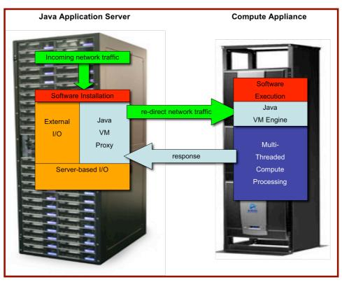
One obvious advantage of this architecture is that the "host" Operating System still appears to be performing the same functionality as before, running the business Application. However, the actual CPU processing is being off-loaded to the Azul machine.
